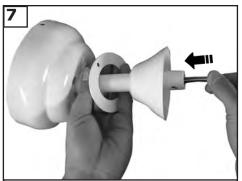
Place canopy, canopy ring and then yoke cover on downrod. Thread leadwires and safety cable through downrod. As shown.
